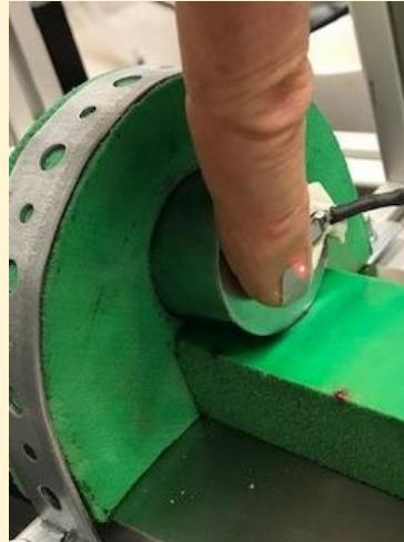
**Measurement of vibration transmission into finger**
